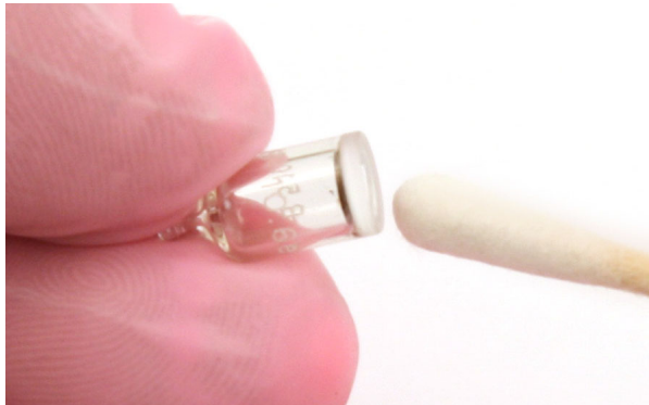
Figure 9: Polishing the Electrode Lamp Window
